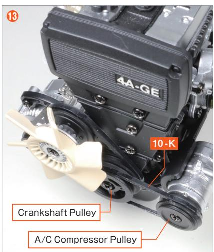
While slightly stretching the **A/C Compressor Belt 10-K**, fit it into the grooves of the **Crankshaft Pulley** and **A/C Compressor Pulley**.
